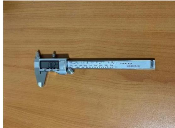
Figure 2. A digital vernier caliper used to measure physical assessment by a tester for criterion validity of the 3D scanner equipment.
