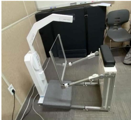
Figure 1. A 3D scanner (MediAce Scan, MS320A) with a lower extremity holder, an acrylic footplate, a scan arm, and a scanner body.
